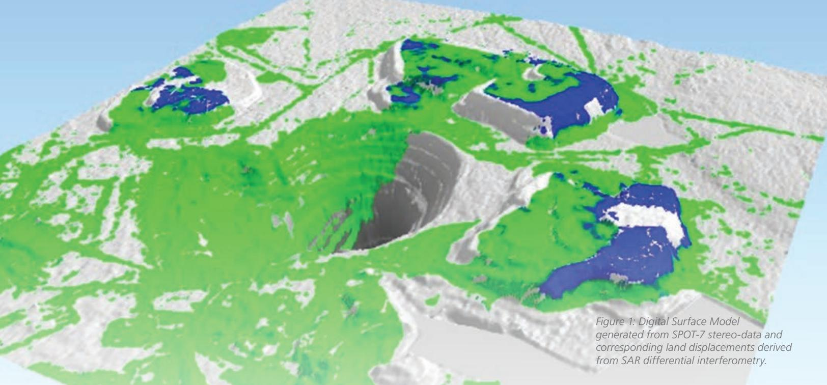
Figure 1: Digital Surface Model generated from SPOT-7 stereo-data and corresponding land displacements derived from SAR differential interferometry.
