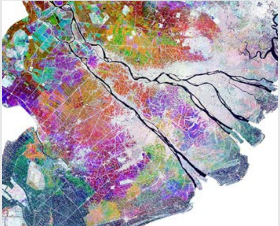
This multi-temporal false color composite of the Mekong River, located in Southeast Asia, shows different stages of crop growth. The source image is Sentinel-1, processed using ENVI SARscape by sarmap SA.
