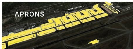
AMDB layers are derived from satellite imagery which has been georeferenced using survey ground control points. Key airport features are digitized from the georeferenced imagery, resulting in location-specific point, line and polygon vector feature classes.
