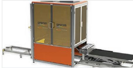
Measure the distribution and quantity of the content of drill cores and other geological samples.
